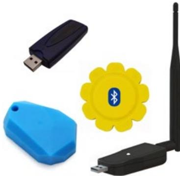
A beacon is a wireless device, usually the size of a watch or pen drive, capable of transmitting periodically a certain signal with minimal power consumption. The typical signal range is around 100m, while long range devices can reach up to 1km. Depending on the signal strength and transmission frequency the beacon can work autonomously for several months or years, without recharging the internal battery. Some beacons rely on USB power instead of internal battery.
